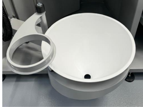
Fig. 19: Powder bag cone complete
