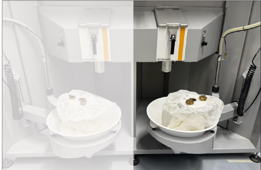
Fig. 97: Placing fresh powder - working area 2
