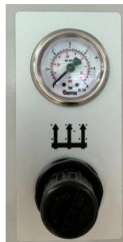
Fig. 11: OptiSpeeder indicator fluidization
