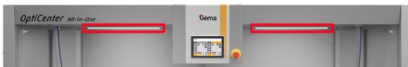
Fig. 8: Status lights-Installation location
