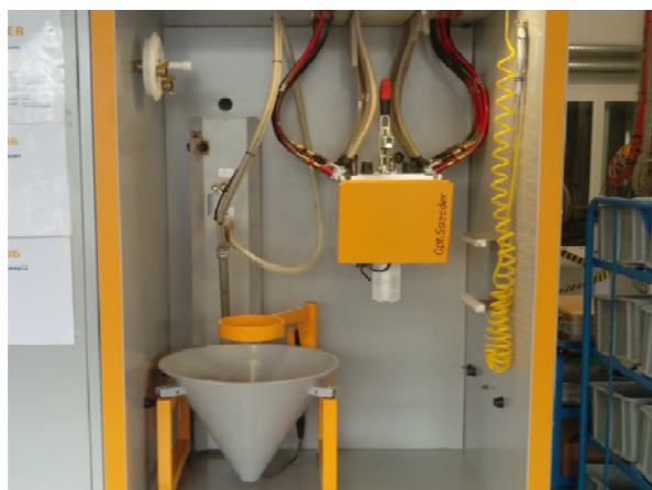
21. Remove powder bag, clean the OC thoroughly
