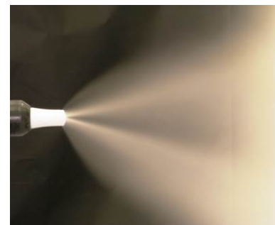
too much electrode rinsing air
