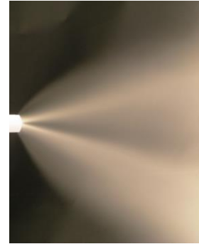
too much electrode rinsing air
