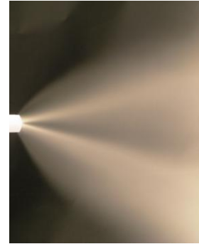
too much electrode rinsing air
