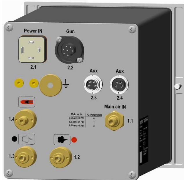
OptiStar CG08-C – Connections - Compressed air hoses / cables
