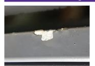
May I please have your opinion as to whether or not the cause of the blistering in this image of powder coated aluminum shutters is likely due to poor or defective pretreatment?
