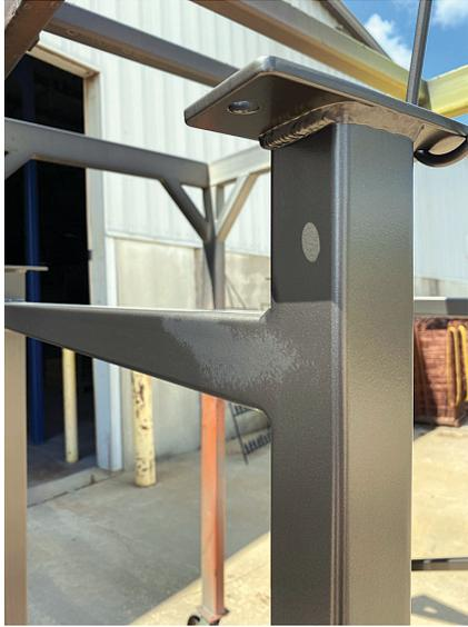
is coming out blotchy around some of the welded joint areas after curing, but also shows up in some of the straight areas of the tubing. We did prime these parts with a gel cure and neither the substrate nor
