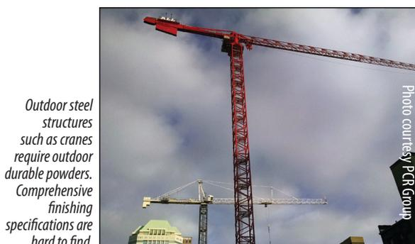
Outdoor steel structures such as cranes require outdoor durable powders. Comprehensive finishing specifications are hard to find.
