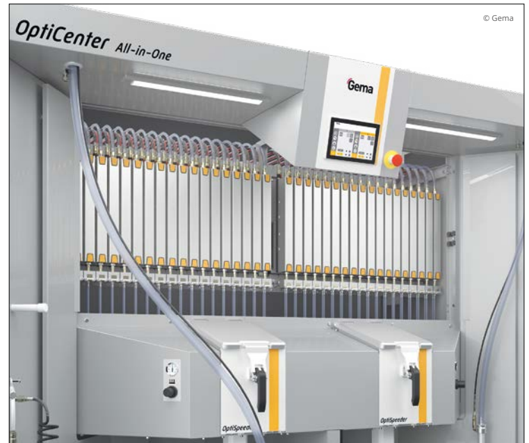
Space-saving integration of the new OptiSpray All-in-One application pumps.
