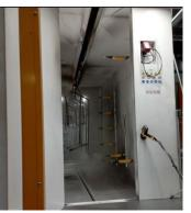
**The UA axes** have made it possible to automate the positioning of the 6 fix guns, by setting up specific programs. This drastically reduces manual pre-touching and achieves high application quality. Operators now work in a more comfortable and safer working environment. 8 months of the year the line works in double shift at 8h and in the rest of the time in single shift.
