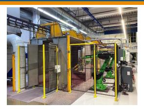
After the expansion in 2020, MWN planned a comprehensive retrofit of the MagicCylinder system from 2002. The goal was to reduce color change times, free up personnel capacity, and increase and stabilize the coating quality. For this purpose, new ZA and XT axes with tilting function to compensate for sloping components, an OptiCenter OC07 powder center with AP01.1 application pumps and the MagicControl 4.0 CM40 control system with GemaConnect were installed on the MagicCylinder.
