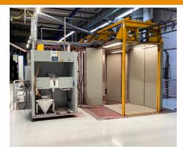
In a second construction stage, the downstream manual coating booth was equipped with two CMA robots during operation and connected to the new OptiCenter OC07. MWN never had to interrupt production during the entire rebuild.
