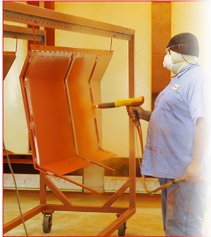
A Flory Industries employee manually applies powder to parts using Gema guns.
