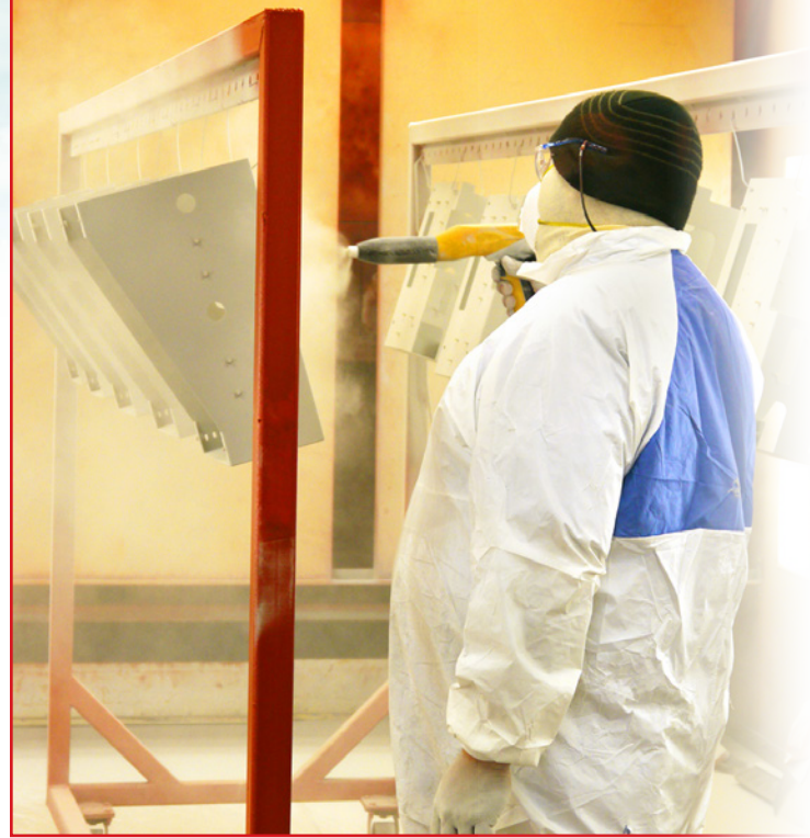
Flory expects to reduce its VOC emissions by 90 percent this year, since installing its new powder coating line.
