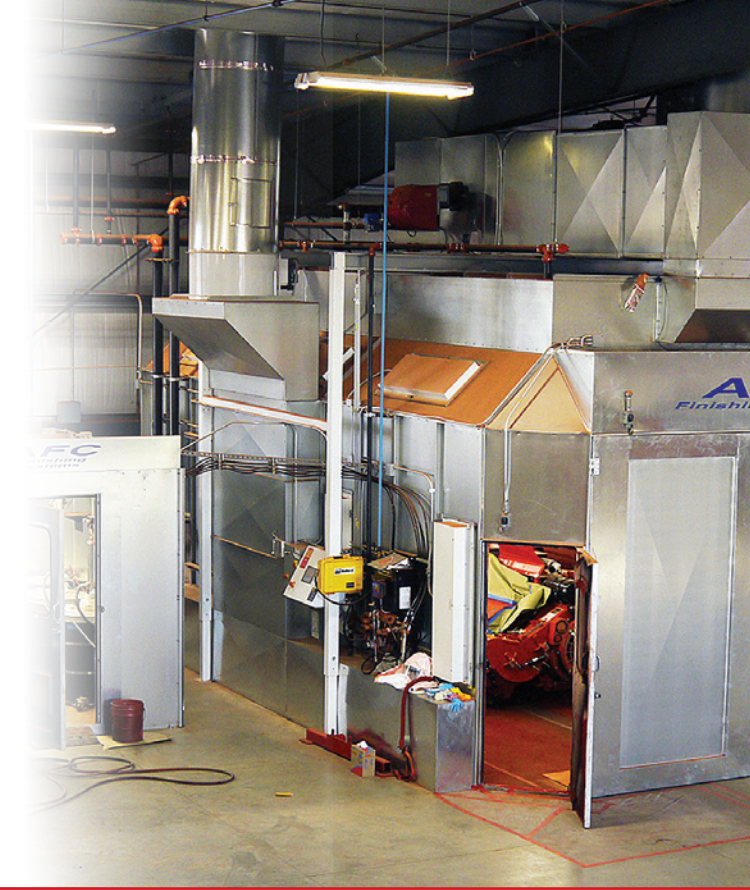
Parts at Flory Industries are dried/prebaked and cured in one of two 12-ft x 30-ft x 10-ft batch ovens.
