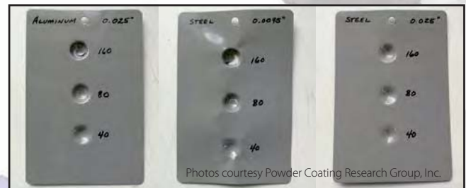
These figures show the impact in inch-lbs. comparing steel and aluminum in various gauges.
