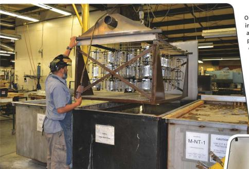
One finishing improvement implemented earlier this year was a conversion to zirconium-based powder coating technology for cleaning and pre-treating metal before powder coating.
