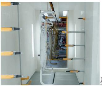
A newly developed gun axis is the ideal solution for coating the insides of housings and complex parts. This system automatically positions each individual gun vertically.
