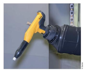
The robotic guns produce a consistent, reproducible coating.
