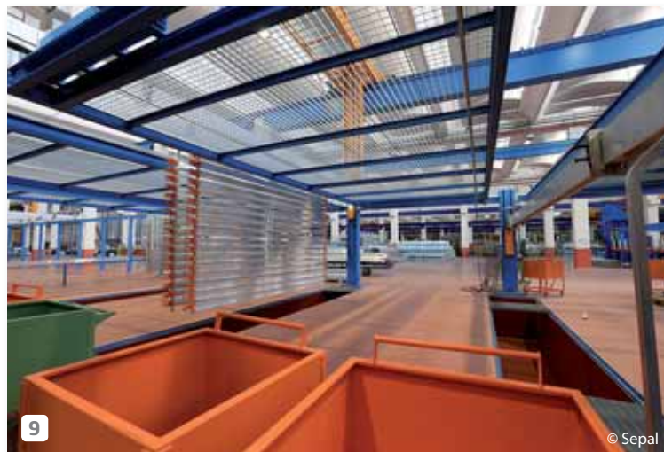
9 The loading area of the oxidation plant.
