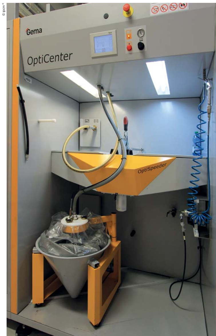
The Gema Opticenter powder management unit with dense phase feed pumps.
