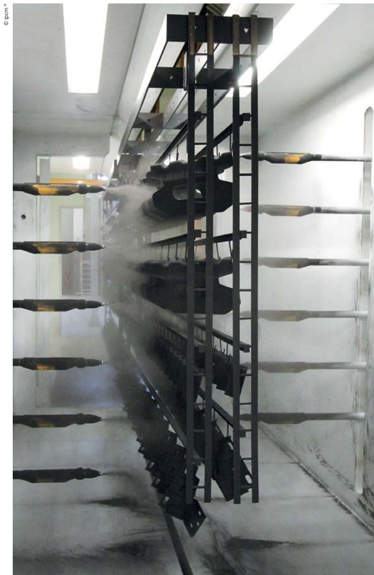
One of the two automatic powder application booths, each equipped with 2 reciprocators and 6 guns per side.
