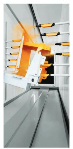
Gema's Dynamic Contour Detection technology uses laser scanners to gather information about the object to be powder coated and then uses that to move each spray gun into the correct position to ensure complete coverage, even in difficult-to-reach areas.
