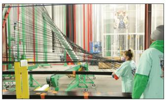
Figure 3. Personnel at the Garden City plant monitor the coated extrusions as they come off the new CUBE vertical powder coating line.
