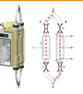
Step 2 – Transfer Transport air pushes powder from the alternate chamber to feed location
