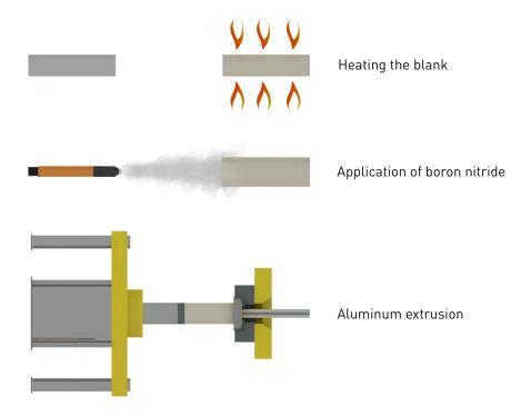
The use of boron nitride is important during the extrusion process of aluminum. Applying boron nitride increases the efficiency and quality of the process. The durability of the die can be increased by the use of boron nitride.
