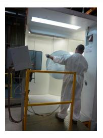
Thanks to the effectiveness of automation, reproducible quality and productivity, manual errors are avoided and re-coating reduced. The level of scraping, offers a lot of powder savings and better thickness consistency (from 75-200  $\mu$ m to 75-100  $\mu$ m). Only 2 operators are now needed for touch-up. In addition thanks to the quality of the automatic color changes, the waste powder loss is reduced by 75%.
