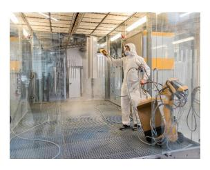
efficient double-cyclone and end filters, fulfilled the challenging demands of Wesemann exactly. The OptiStar application control with PCC Mode is ensuring a high penetration with soft powder cloud. A wide space glass booth for manual special coating is placed parallel and equipped with an OptiFlex2 B manual coating system.
