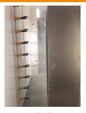
programme they have recently installed a new automatic Gema Magic Compact powder coating plant.
