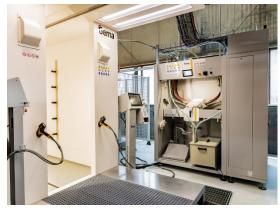
critical areas if necessary. All coating processes are controlled centrally via the MagicControl 4.0 control system. The waste powder is collected in a BigBag.
