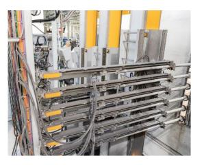
stored programs. With a new component, the operators have to replace the flat-jet nozzles with angle nozzles at most. To optimize powder output, BIRN uses the OptiCenter® powder centre with AP01 pumps.
