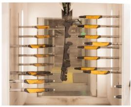
change to cathodic dip coating (CDC) combined with powder coatings.
