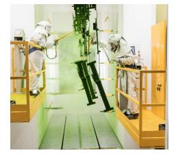
Not unlike the agricultural machinery produced by Amazone, the new unit is designed for maximum efficiency. Precise gap control, axis with angled guns, vertically adjustable manual coating stations, the full recovery of powder and a power circuit for electrical loads. The overall package supports efficient and high-quality coating.
