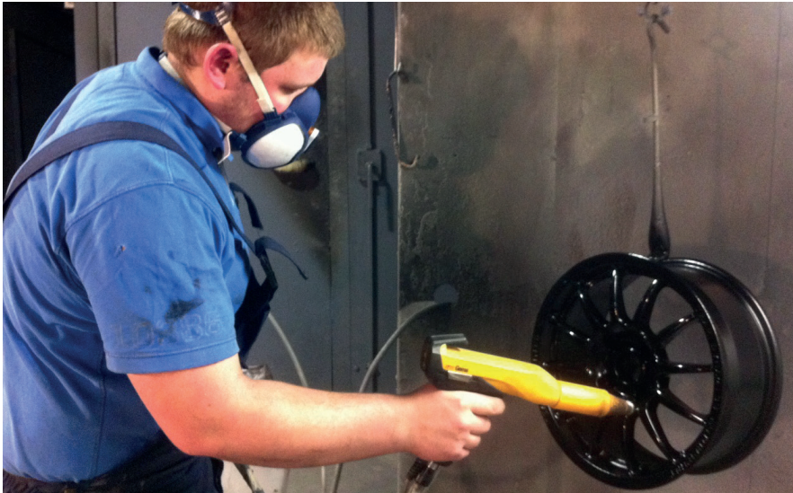
Darren Burgess the Operator is applying a custom colour to mini cooper wheels for «Team Steigh Racing» a local race team sponsored by Pentland.
