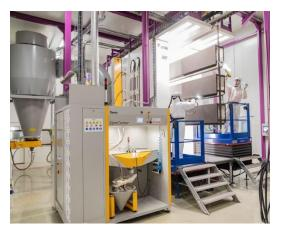
WOB is particularly impressed with the neatness of coating surfaces and the high level of automation. The ambition of having "1 program for all parts" was implemented from practically the begin. With two post-coating unit stations on elevating platforms, WOB is able to work with great flexibility, achieve outstanding quality levels, and ensure faster throughput rates. There has also been a massive reduction in the rework associated with the complex diversity of parts.
