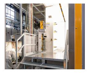
and cabin technology in a new building at the company's headquarters in Gutersloh. In order to coat as wide a range of parts as possible, the EquiFlow color-change system from Gema has especially large openings. The OptiCenter OC08 with injectors was first used at the Helling & Neuhaus facility. Combined with the CM40 control system, the new coating system offers a very high level of automation.
