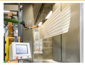
The family-owned company Kurt Opfer Oberflächenschutz from Mudersbach, Germany, has been using two robots for automatic coating for many years. Instead of manual coaters, these robots carry out pre- and post-coating in a MagicCylinder QCS01 with central medium extraction. As a result, high-quality coating results have always been achieved in automatic mode, with the robots and during manual coating.
