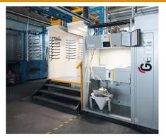
brand new **Gema** boothsystem with all the latest equipment and **Smart Inline Technology (SIT) pumps.** As well as **OptiCenter OC07** for quick color changes and a MagicControl CM40 with all the latest 4.0 industry updates. Target of the installation were: improving coating quality, powder savings and increased conveyor speed from the 2 m/min to the actual 3.6 m/min. In a recent interview published in the magazine **IPCM**, Fulvio Giordano, owner and founder, expressed all his satisfaction:
