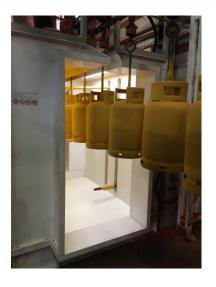
decision to upgrade was a combination of efficiency and health & safety improvements. The system was installed in a very tight space to incorporate the existing conveyor system and oven, this required a custom designed booth with a very low floor to fit in the space required.
