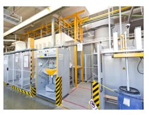
the various part geometries. Gema's installation ensures consistently high quality coating in addition to ease of use, particularly with very regular coat thickness distribution. This is ensured by the application pumps AP01 in the OptiCenter. The quality is so high that Siemens forewent a scheduled, non-contact coat thickness measurement. Thanks to the new electrostatic powder coating system, the busbar distribution systems from Siemens will continue to reliably ensure a modern power supply.
