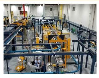
Their decision was to select a system designed and installed by Gema's distributor, Dietz Supply Company. The Gema equipment included in this system were two (2) automatic booths (prime coat and top coat) as well as the replacement of automatic guns used on a chain-on-edge line (clear coat.) The results have been extremely successful as they are experiencing increased production throughput and operational efficiency, along with outstanding coating performance.
