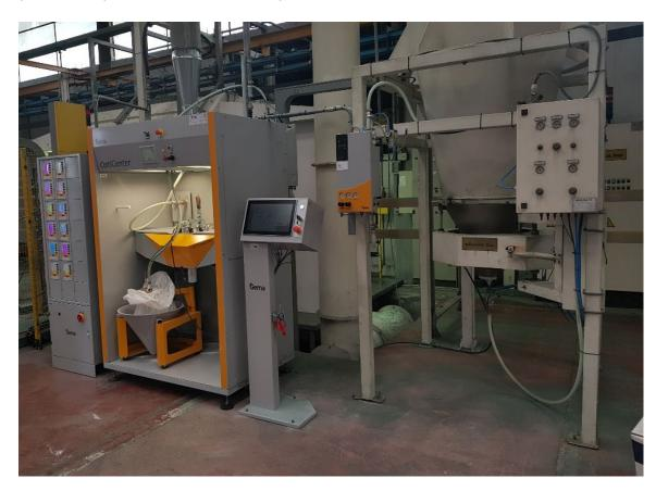
The continuous research of Italver to the highest quality possible has pushed the owner Mr. Massimo Gasperi to try the advantages of the dense phase application technology (OptiSpray) with the APO1 application pumps produced by Gema. This factor led him to replace the traditional old equipment with venturi pumps with the dense phase application system, including a gap control system and the new control master *MagicControl 4.0, CM40* to monitor and control every application aspect.
