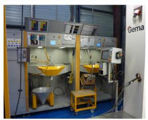
French well-known а aluminum profiles' job coater, which vertical lines are equipped with Gema's automatic guns. In 2015, it and contacted us our main competitors to for 2 new powder lines, dedicated to very small series and profiles particularly difficult to paint. Special goal for these new lines: Changing color in 6mn maximum. In order to win the order, our Suisse engineers adapted the existing MultiColor Switch to customer's needs. So finally, we installed
