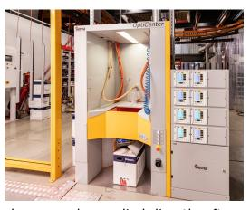
layer can be applied directly after the first one without heating the parts in between. This saves one oven and one cleaning cycle. This way Trioliet consumes the equivalent of 75,000 m<sup>3</sup> less natural gas per year! At the same time the production capacity has been doubled with the new Gema plant. This shortens the throughput time and reduces energy consumption by 50% compared to similar plants. Trioliet thus has one of the most environmentally friendly coating lines in the world.
