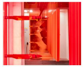
edges and corners explicitly require a double coating which consists of a primer and a top coat. Together with Gema Switzerland GmbH and AkzoNobel Powder Coatings, Trioliet developed a new "Dry on Dry" double powder coating process for this purpose – it is to date unique worldwide.
