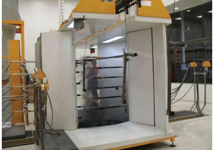
Powder application is via 12 automatic guns mounted on oscillators. Touch-up stations at each end of the booth are rarely used.
